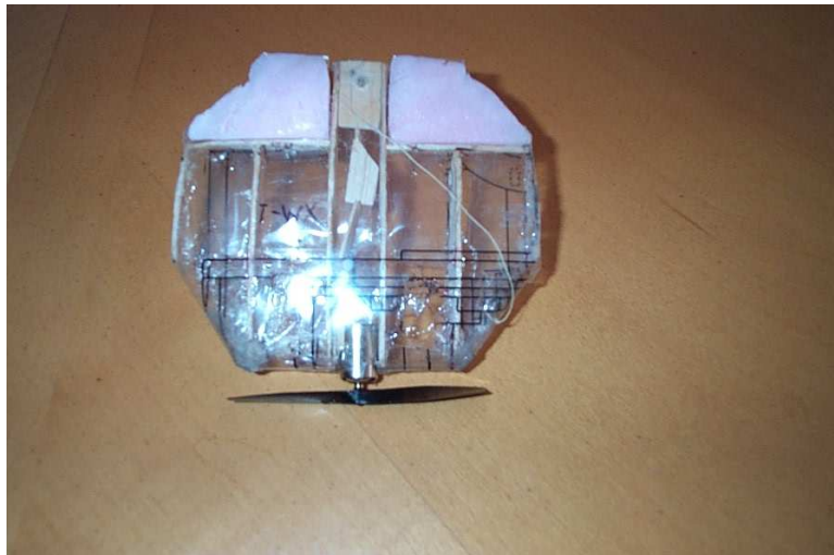
Figure 3: Full Airfoil — Balsa and Transparency Constuction
